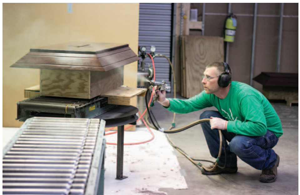
▲ Top: Eric Boeglin assembles a casket lid. Below: Ross Tempel sprays the top coat onto the lid of an Abbey Casket.
